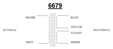
Looks to be 8 ohms / 100V line, 100 Watts with an additional monitor winding. Turns Ratio of Pri:Sec 1 is 1.37 and Pri:Sec2 is 1:0.47
