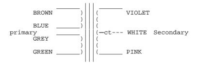
600ohm /600ohm, turns ratio 1:1, max level 2.75Vrms at 30Hz. With electromagnetic shielding (mumetal can), Quadrifilarly wound for best h/f response. Frequency response on a measured sample was -ldB, 10Hz - 120kHz, with source and load both 600ohm and input voltage 0dBr.
