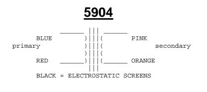
200 ohms primary. 5k ohm secondary. Turns ratio 1:5. ±1dB 20Hz-20kHz. Max level 2V at 30kHz. Electrostatic screens. Mumetal can. style f (Two M3 threaded holes 19mm apart for mounting. Flying leads exit at side of can.)
