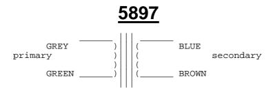
Transformer for tape head , 10 ohms and 7mH. Step up turns ratio 1:4. Frequency range 30Hz-20kHz. Input volts at 30Hz=0.5mV.
