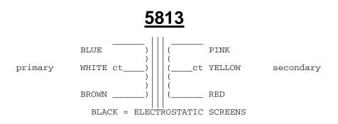
10kohm/10kohm, turns ratio 1:1, max level 9V rms at 30Hz. With electrostatic and electromagnetic screening (mumetal can) Transformer is bifilarly wound for best CR balance. Frequency response on a measured sample was -1dB, 20Hz - 30kHz, with a source of 2kohm and load of 600ohm and input voltage 0dBr.
