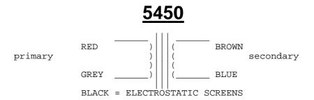
Turns ratio 1:2.25 Frequency response +/- 0.5dB 20hz - 20kHz Maximum level 1.35Vrms at 30Hz. Electrostatic and electromagnetic screening.
