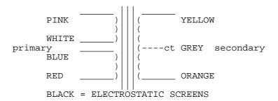
200 ohms microphone transformer. 1:5 step-up ratio (in series). 5k ohms load.
