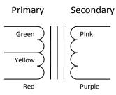
Further Information: Ratio – 1CT:4 ( $600\Omega/10k\Omega$ ) Frequency Response: +/-1dB, 20Hz-20kHz (Z<sub>Load</sub> =  $600\Omega$ )
