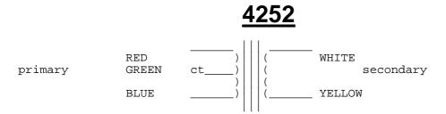
Microphone transformer. Primary 200 ohms centre-tapped. Secondary 200 ohms. Turns ratio 1:1. Frequency range 20Hz-20kHz +/-1dB. Level 1-5V at 30Hz. In a mumetal can 34mm x 24mm with two tapped holes for fixing.
