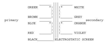
600 ohms/600 ohms Both primary and secondary are brought out in two halves which can be connected In series for 600 ohms or in parallel for 150 ohms. With electrostatic screens.
