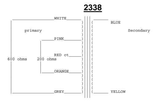
This is basically our Standard Multitapped Microphone Matching Transformer Type 3678 (see data sheet for specification) but with centre-tapped primary and  ${\bf NO}$  30 ohms tap
