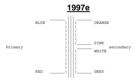
**1997e 200 ohm 2-way splitter combiner** 3 x 200 ohm windings. As 4297 but has no centre taps.
