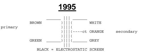
This is a modification of Sowter type 8055 cartridge transformer. Turns ratio has been altered to 1:32 by reducing Primary turns as requested.
