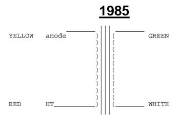
1985 Single Ended triode to line output type 9040 Modified for 2:1 Step-down Ratio as Requested – keeping the original Primary.
