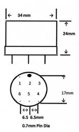
This is type 3575 with pcb pins and OCC wire
