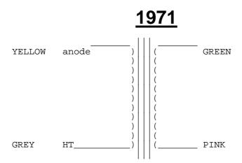
1971 Single Ended triode to line output type 9040 Modified for 2:1 Step-down Ratio as requested.
