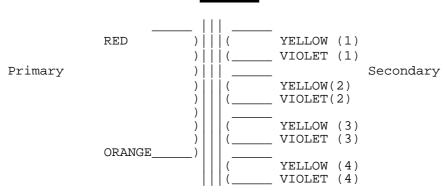
There are FOUR EQUAL SECONDARY WINDINGS which can be arranged for loads of 1, 4, 8/9 or 15/16 ohms thus:-
