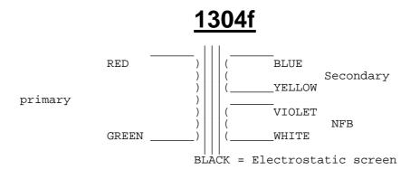
12.1 dBu AUDIO TRANSFORMER type number 1304 Similar to Neumann U67 as discussed with Brian Sowter Primary impedance 9800 Ohms. Secondary impedance 200 Ohms. LF Cut off -0.5 Db at 20Hz. Source 2000 Ohms Turns ratio 7:1 (nfb approx 33% of secondary) with electrostatic and electromagnetic screening. Mumetal Can 34mm diam x 24mm high with 2x M3 threaded holes at 19mm centres for mounting (screws should enter transformer maximum 3mm) Colour coded leads.
