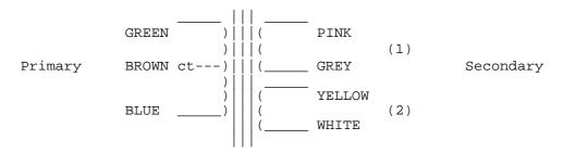
Join two secondaries in parallel for 10:1 ratio or in series for 5:1)
