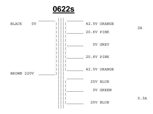
\* FOR PRIMARY WINDING WITH SOLID CORE WIRE AND SLEEVING The solid wire inside the sleeving is coated with polyurethane and needs to be stripped away and tinned if the leads are shortened. For secondary windings with solid core leads please follow the same process.
