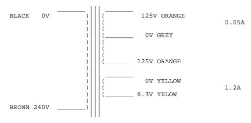
\* FOR PRIMARY WINDING WITH SOLID CORE WIRE AND SLEEVING
