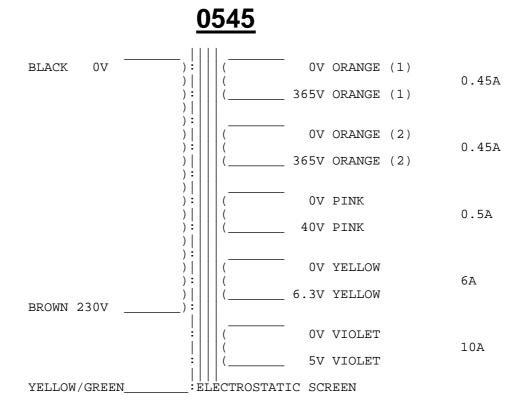
FOR FLEXIBLE LEADS PRIMARY - just cut short and isolate (INDIVIDUALLY) any spare connections
