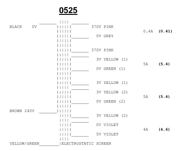
\* FOR PRIMARY WINDING WITH SOLID CORE WIRE AND SLEEVING The solid wire inside the sleeving is coated with polyurethane and needs to be stripped away and tinned if the leads are shortened.
