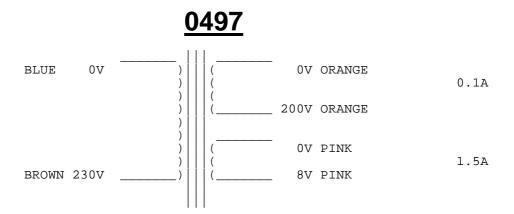
\* FOR PRIMARY WINDING WITH SOLID CORE WIRE AND SLEEVING The solid wire inside the sleeving is coated with polyurethane and needs to be stripped away and tinned if the leads are shortened.
