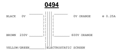
$\underline{*}$  FOR PRIMARY WINDING WITH SOLID CORE WIRE AND SLEEVING The solid wire inside the sleeving is coated with polyurethane and needs to be stripped away and tinned if the leads are shortened.
