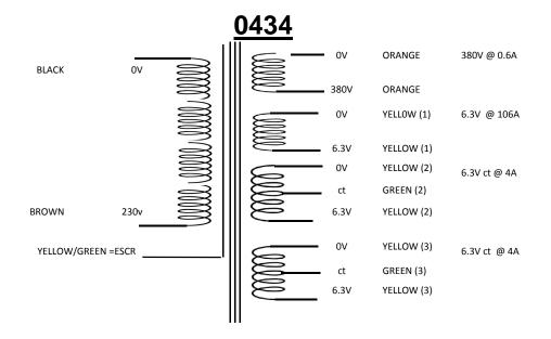
NOTE: A certain amount of mechanical hum is prevalent in mains transformers and can be amplified when bolting to your metal work. Therefore you may find a small rubber gasket or similar material is worth fitting to quieten this hum to its' minimum, but please ensure the frame is grounded to the supply safety earth.
