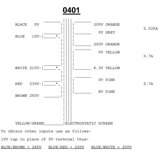
\* FOR PRIMARY WINDING WITH SOLID CORE WIRE AND SLEEVING You will note that the Primary is built up in sections and the two wires in the Blue, White and Red sleeves must always be <u>individually</u> joined to make the primary circuit complete. Spare connections not required can be cut short, each colour joined separately and isolated. The solid wire inside the sleeving is coated with polyurethane and needs to be stripped away and tinned if the leads are shortened.
