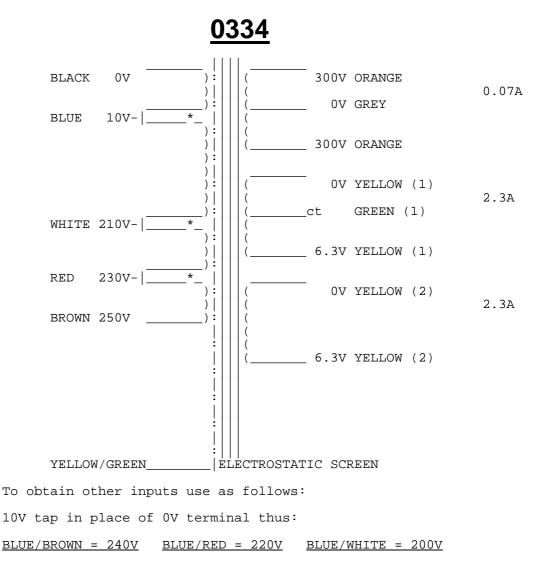
\* FOR PRIMARY WINDING WITH SOLID CORE WIRE AND SLEEVING You will note that the Primary is built up in sections and the two wires in the Blue, White and Red sleeves must always be <u>individually</u> joined to make the primary circuit complete. Spare connections not required can be cut short, each colour joined separately and isolated. The solid wire inside the sleeving is coated with polyurethane and needs to be stripped away and tinned if the leads are shortened.
