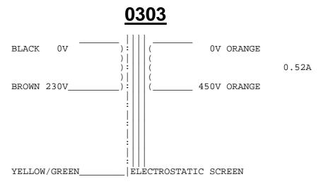
\* FOR PRIMARY WINDING WITH SOLID CORE WIRE AND SLEEVING
