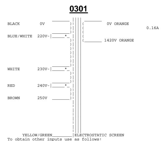
\* FOR PRIMARY WINDING WITH SOLID CORE WIRE AND SLEEVING
