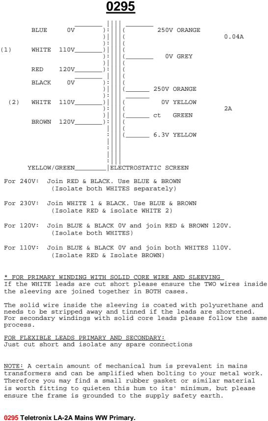
Power transformer for Teletronix LA-2A Compressor. 2 x 120,110 V Primary. 250-0-250 at 40 mA. 6.3V CT at 2 A. Internal electrostatic shield for reduction of noise caused by power line transients. Fully shrouded package. Size "F".
