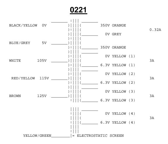
\* FOR PRIMARY WINDING WITH SOLID CORE WIRE AND SLEEVING If the WHITE leads are cut short please ensure the TWO wires inside the sleeving are joined together in BOTH cases.
